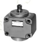
These valves are available either with or without an integral check valve which allows free reverse flow. Flow rate through the valve is regulated by the movement of the spool, which is operated by a cam.
