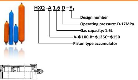
HXQ is an separated accumulator in a hydraulic system, which can store energy of the system and release it when it is needed.
