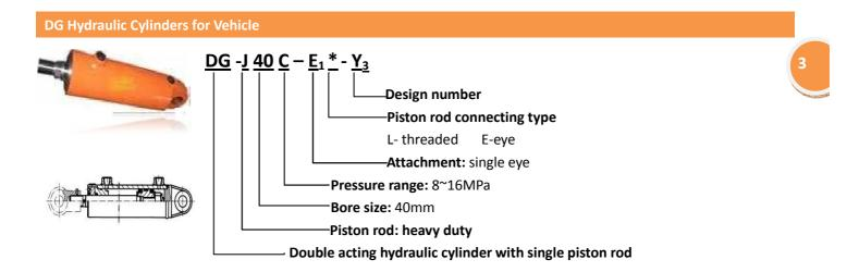
This is a double-acting hydraulic cylinder with single piston rod. Operating pressure is 16MPa, bore from 40 $^{200}$ mm, stroke  $\leq 2000$ mm.
