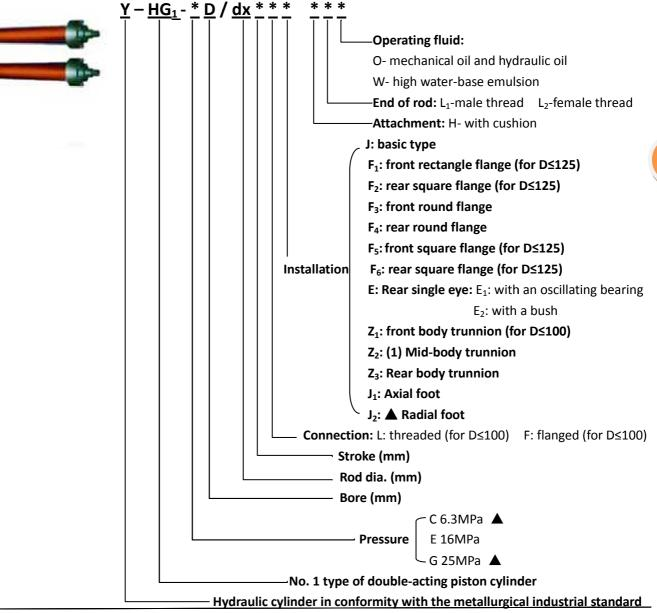
This series cylinder is double-acting piston type hydraulic actuator which can push its piston rod to move in both directions so that its piston will drive other working parts to reciprocate in line. With features, as well as integral damper and air bleeder, it is suitable for metallurgical industry and is in conformity with the specification on mounting and connecting ISO 6020/1 - 1981.
